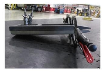
Force to identify non-critical parts that can be replaced using additive manufacturing technology, including a restraint strap for a first aid kit in the B-1 aircraft. In many of these aircraft, the Air Force has experienced failures with original restraint straps, which risks the dislodging of first aid kits during flight. As original replacement straps are no longer manufactured, there is significant costs and wait time produce new parts through traditional means.
