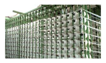
Automatic Sectional Warping Machine (for industrial Fabrics)
